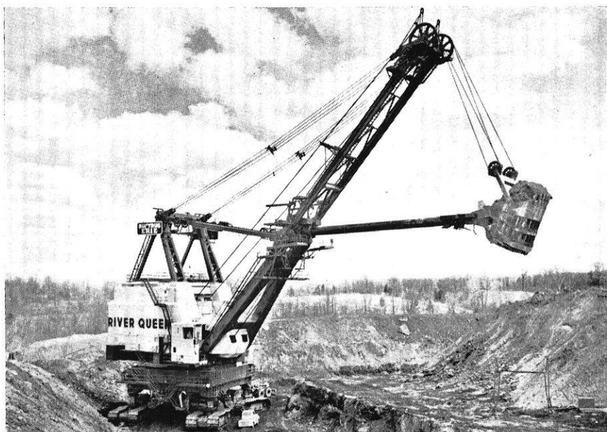
Swinging High! Standing on one seam of coal the River Queen clears limestone overburden from an upper coal seam. Note the pickup truck in the foreground.
