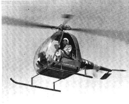
The Army's first operational rotor-tip propelled jet helicopter—built by Hiller.
