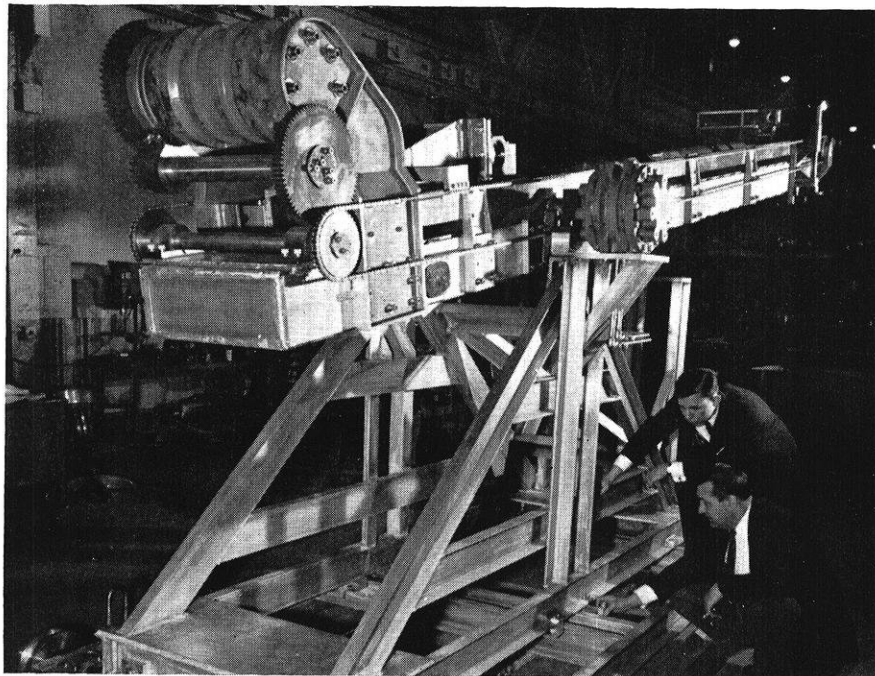
—Photo Courtesy Westinghouse This unique machine will handle radioactive materials under 18 feet of water and will operate on its own small railroad track.
