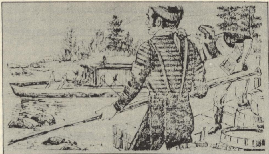
A durham boat could carry 15 to 50 tons of freight. Pointed poles were used to propel the vessel. When water was too deep, a sail was hoisted.
