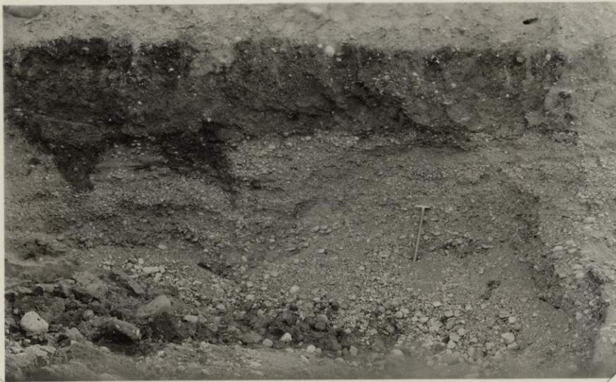
Figure 9. Picture taken with superortho film and K_2 filter. Note that weathered zone is lightened in tone and detail shows well.
