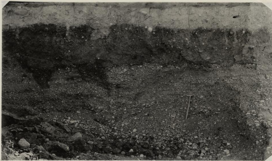
Figure 10. Picture taken with superortho film and C filter (blue). Note that weathered zone is made dark obscuring detail and that the detail of the gravel is better than with the yellow filter of fig. 9.
