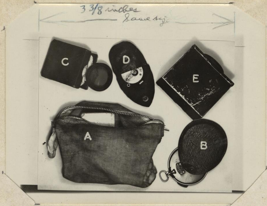
Figure 5.—Field kit of accessories. A = bag with zipper which contains all apparatus. B = a small, and inexpensive exposure meter of the actinometer type. C = filter in metal cell with box and cloth for cleaning. D = self timer. E = lens hood designed by the writer.
