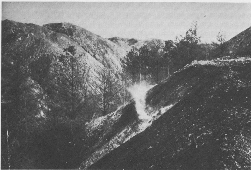
Figure 5.7. A typical self-heating coal refuse pile (right side of picture). This was a pile at the Blackfoot #5 Mine, near Winslow, Indiana, photographed in 1969. Note the smoke and steam. The large pile on the left is not coal refuse, but a spoil bank from the strip mining operation. Spoil banks do not self-heat and are much less acidic.
