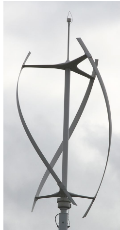
(b) A Gorlov type CFT that has helical blades [7].
