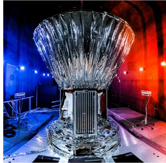
Figure 76 (Left) Overall observatory TVAC chamber layout and temperatures. (Right) Image of SPHEREx with outer Photon Shield blanket in TVAC chamber
