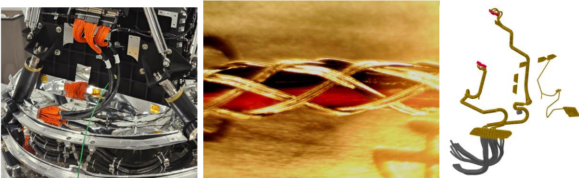
Figure 28 (Left) Image of as-installed SWIR detector harness. (Center) Microscope image showing partial braid coverage. (Right) Representative surfaces in Thermal Desktop
