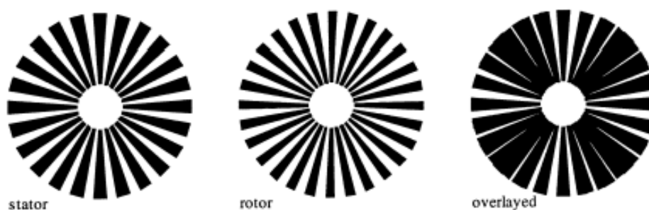
Fig 1.5-7 Graphical representation of the air-gap permeance variation created by rotor and stator slotting (28 rotor slots and 24 stator slots) [163]
