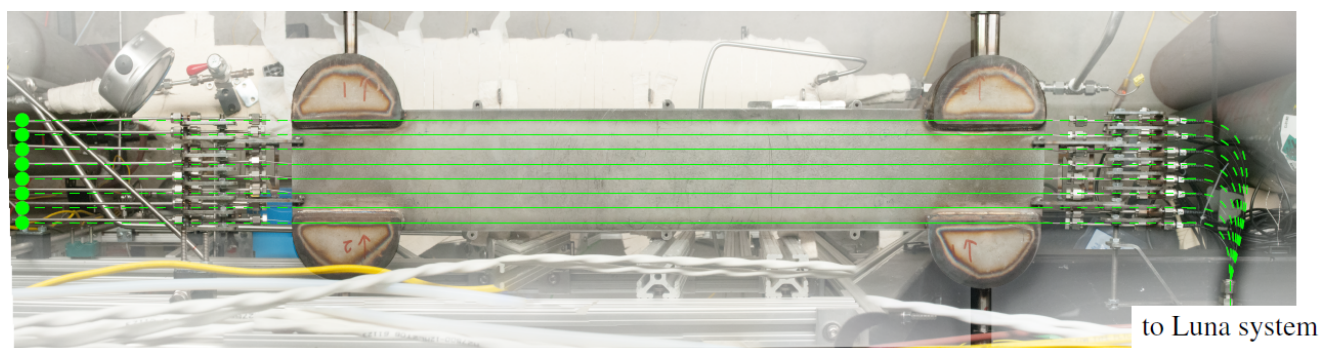
Figure 6.4: Fibers instrumentation of Airfoil recuperator, solid lines are region of measurement
