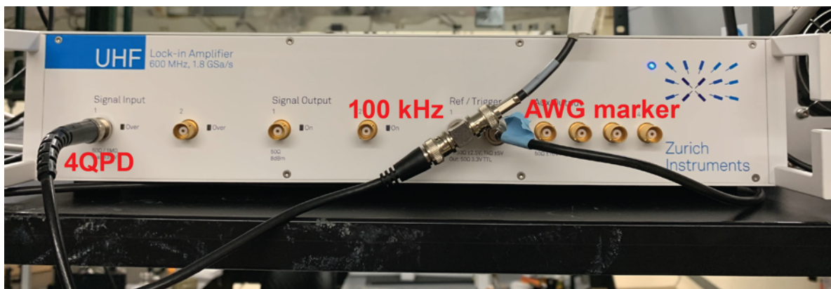
Figure 2.10. Zurich Instruments UHFLI used for the FTPT experiments. The left most input is the 4QPD signal. The first trigger, shown in trigger input one with a T-joint, is the 100 kHz trigger from the laser electronics. The second trigger, the furthest on the right, is the trigger marking the beginning of each mask sequence from the AWG.
