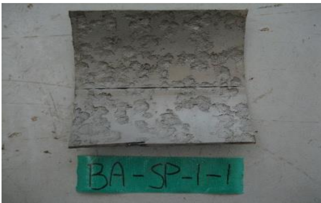
Figure 3.20. A pipe sample of a 200-mm diameter steel water main after sandblasting for pipe cleaning.
