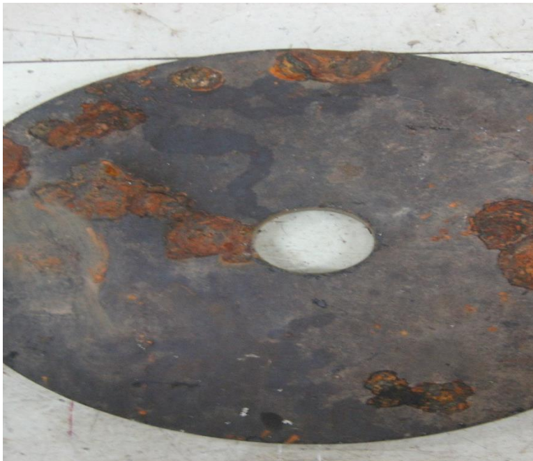
Figure 3.13. A pipe sample of a 1,650-mm diameter steel WTM before sandblasting for pipe cleaning
