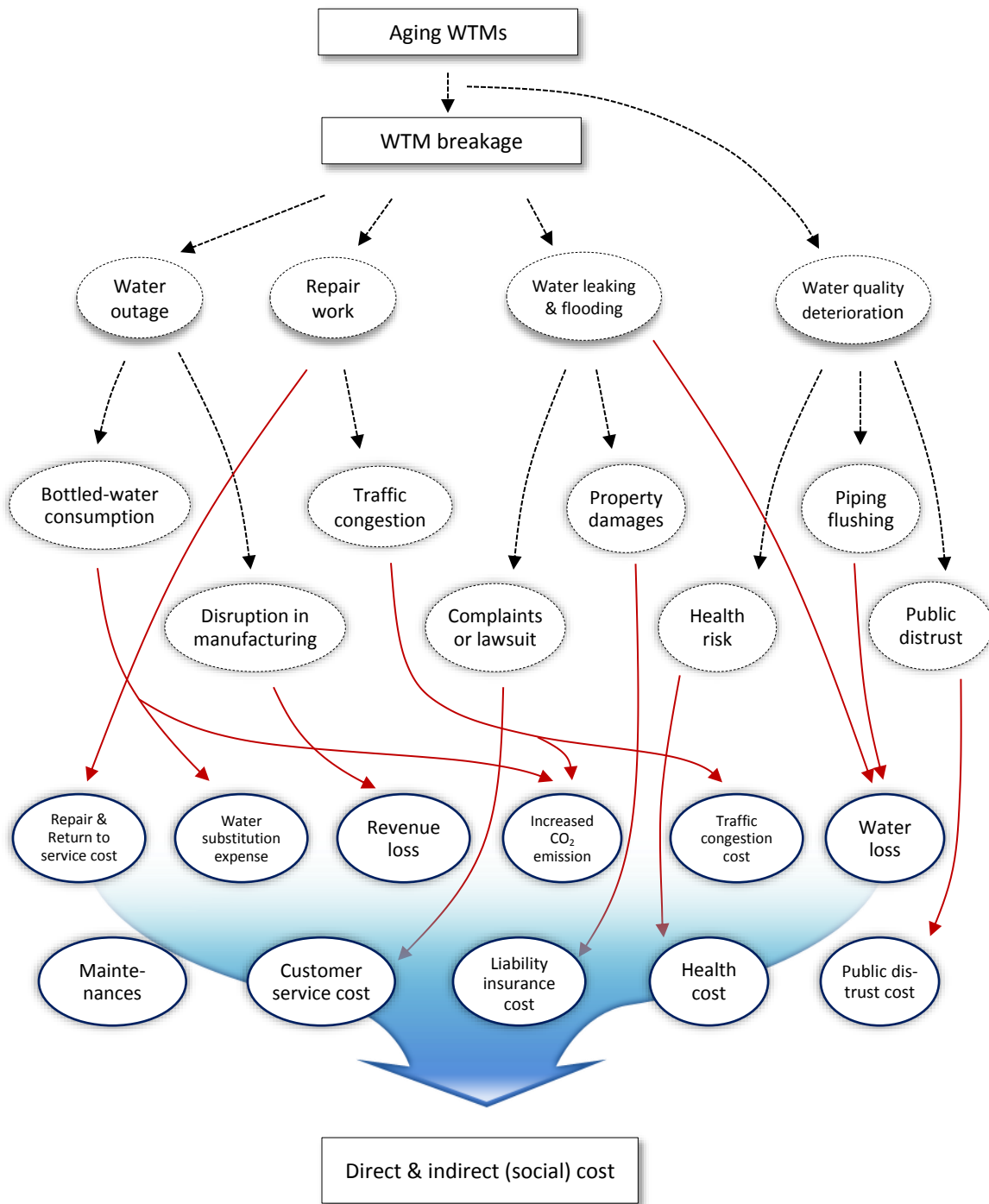
Figure 5.2. Schematic of the damages and costs caused by breakage and deterioration of aging pipelines
