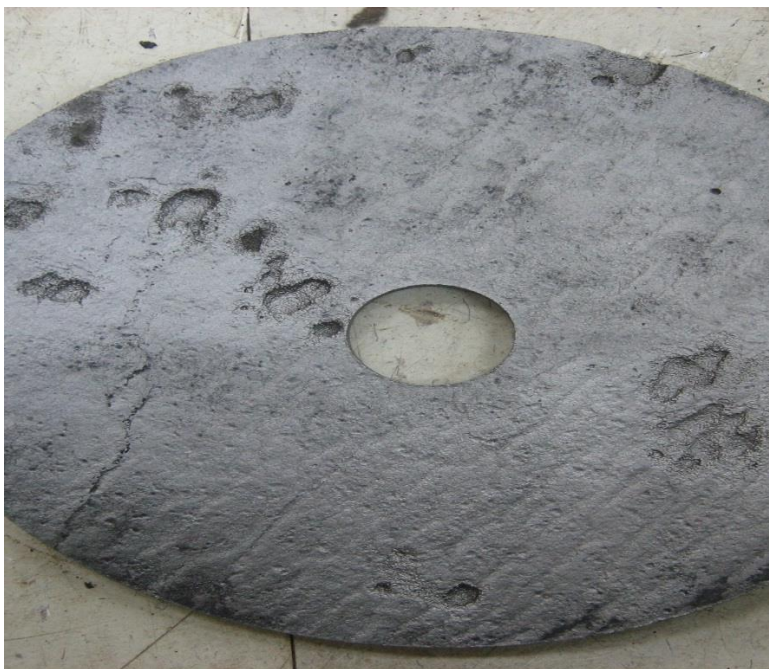
Figure 3.14. A pipe sample of a 1,650-mm diameter steel WTM after sandblasting for pipe cleaning.
