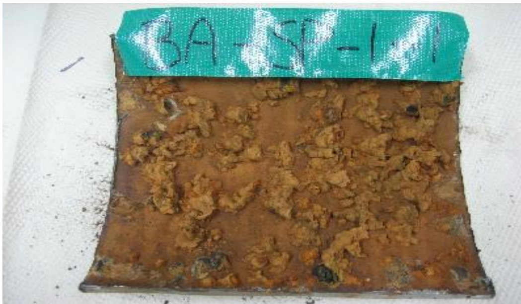
Figure 3.19. A pipe sample of a 200-mm diameter steel water main before sandblasting for pipe cleaning
