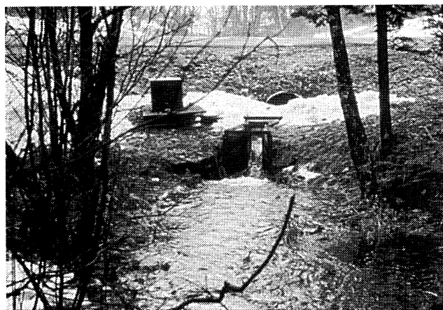
Parshall Flume and stage recorder at inlet 1 of Lake Clara during snowmelt runoff — view upstream of the lake.
