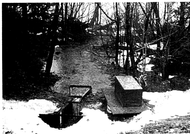
Parshall Flume and stage recorder at inlet 1 of Lake Clara during snowmelt runoff — view downstream from County Highway A.
