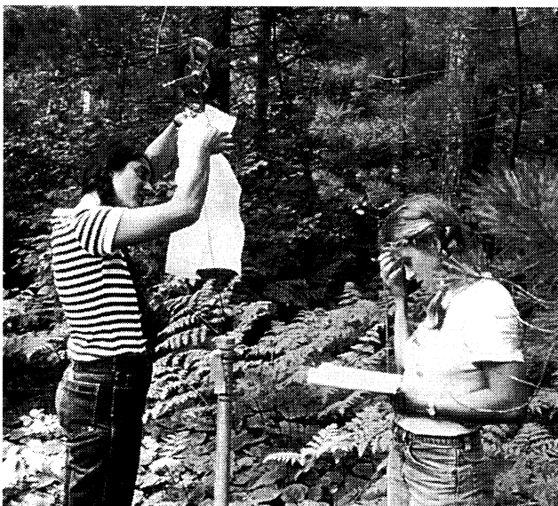
DNR field assistants Nan Eckert and Lisa Huberty determining water table depths in a groundwater piezometer at Lake Clara.
