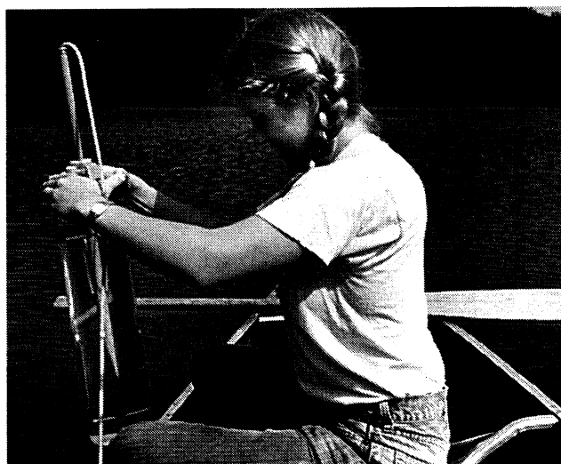
DNR field assistant Lisa Huberty using a Kemmerer sampling bottle to collect water samples.
