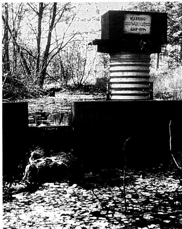
Recording V-notch weir at the outlet of Lake Clara.
