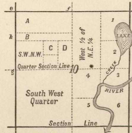
In the subdivision of quarter sections, the quarter quarter corners are to be placed at points equidistant between the section and quarter section corners and between the quarter corners and the common centre
