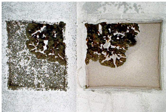
Figure 5. Agar and bacterial colony on glass slide with matrix applied via dry sieve (left) and TM-Sprayer (right).
