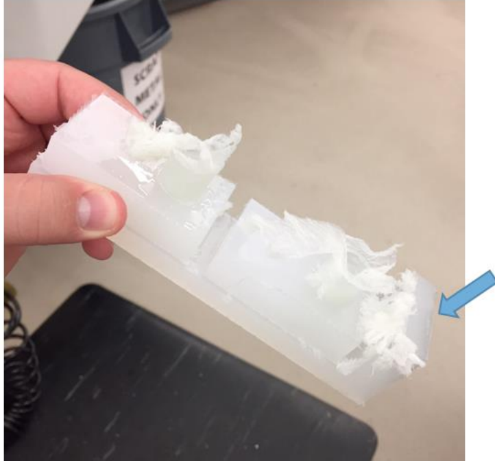
Figure 7.3: Full piece after Operation 1 with part that needs to be trimmed indicated (arrow)
