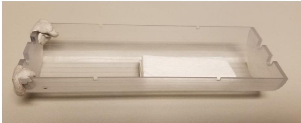
Figure 7.24: Bioreactor tray with paper towels inside to support the bioreactor during experiments.
