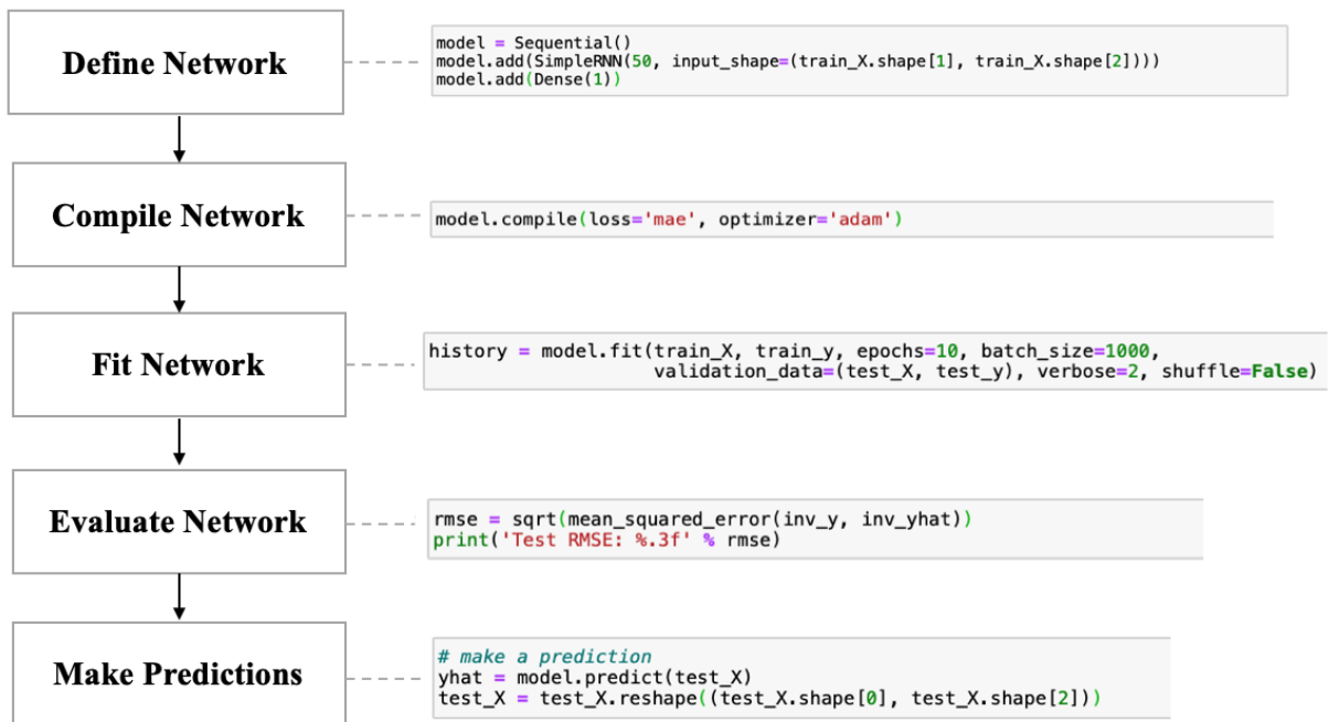
Figure 4.9 Five steps to develop a simple RNN model.
