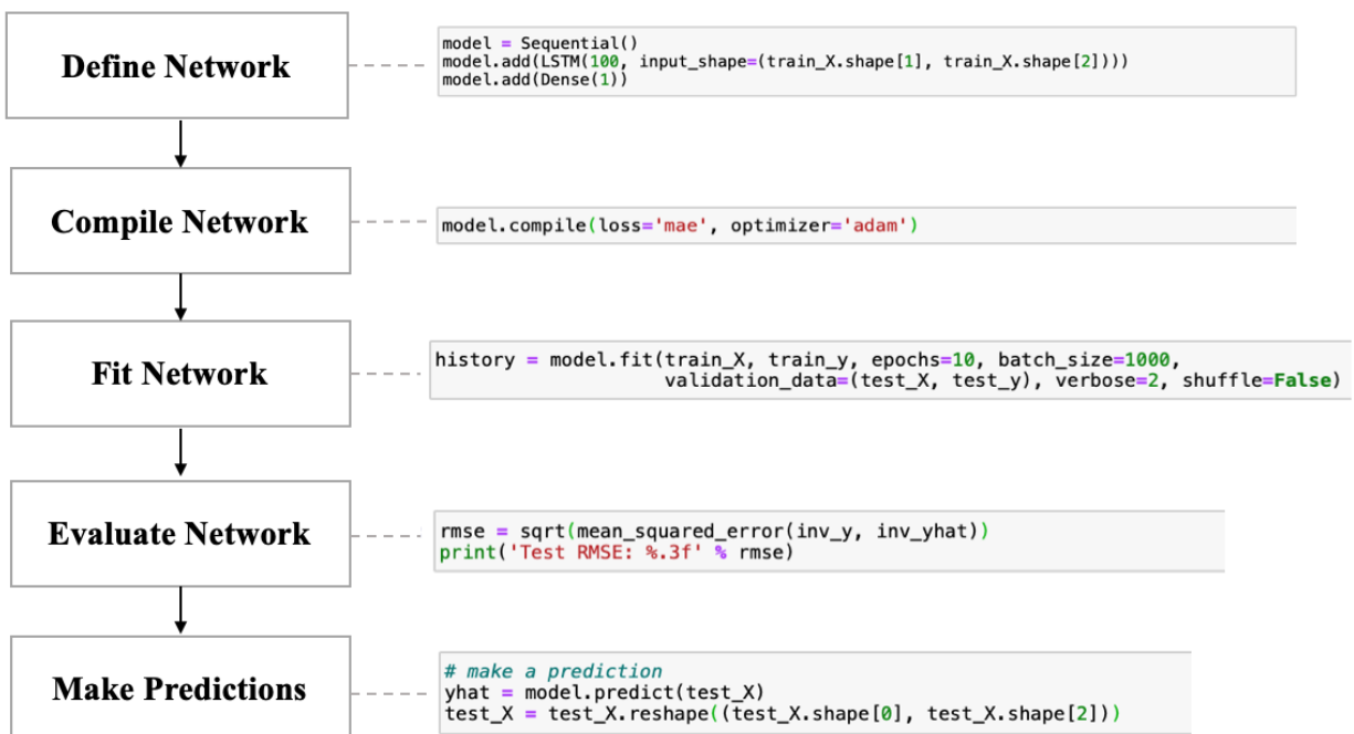
Figure 4.10 Five steps to develop an LSTM model.
