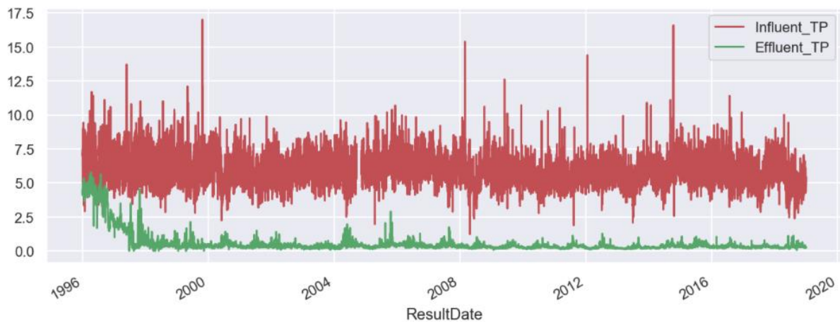
Figure 3.9 The relationship between influent and effluent in TP.
