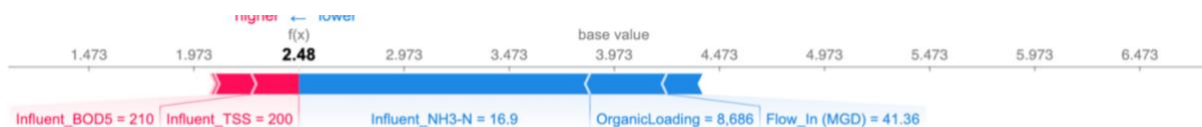
Figure 5.16 The force plot of the first observation including flow rate and organic loading.
