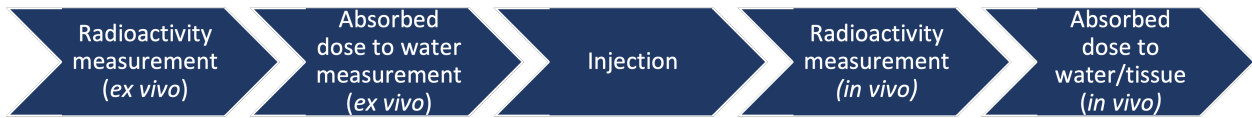
Figure 2.16: The proposed workflow for TRT treatments establishes ex vivo absorbed dose traceability.
