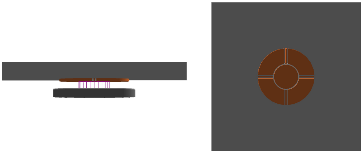
Figure 5.15: The graphics rendering of the PCB EC in TOPAS MC code. The left figure shows the XZ view of the PCB and the source substrate. The right figure shows the XY view of the PCB without the presence of the substrate.
