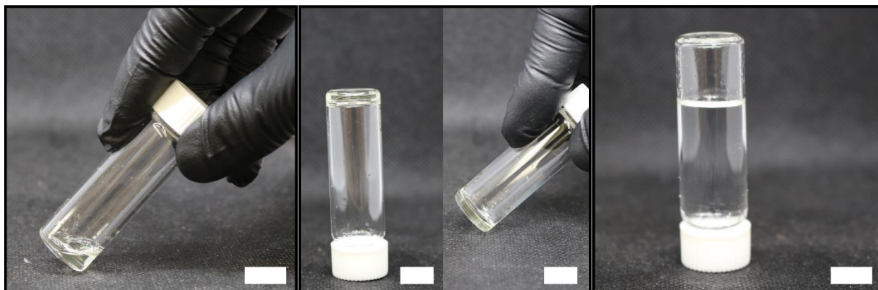
Figure A13A. Left) Liquid 4-pGA-3 resin prior to light exposure. Middle) 4-pGA-3 resin after light exposure held upside down and at an angle. The resin solidified and no longer flowed. Right) Solidified resin after being dissolved in dichloromethane. It no longer adhered to the bottom of the vial and dissolved in solvent. Scale bars indicate 10 mm in each image.
