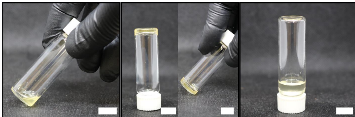
Figure A13B. Left) Liquid SMA-3 resin prior to light exposure. Middle) SMA-3 resin after light exposure held upside down and at an angle. The resin solidified and no longer flowed. Right) Solidified SMA-3 resin after being dissolved in dichloromethane. It no longer adhered to the bottom of the vial and dissolved in solvent. Scale bars indicate 10 mm in each image.
