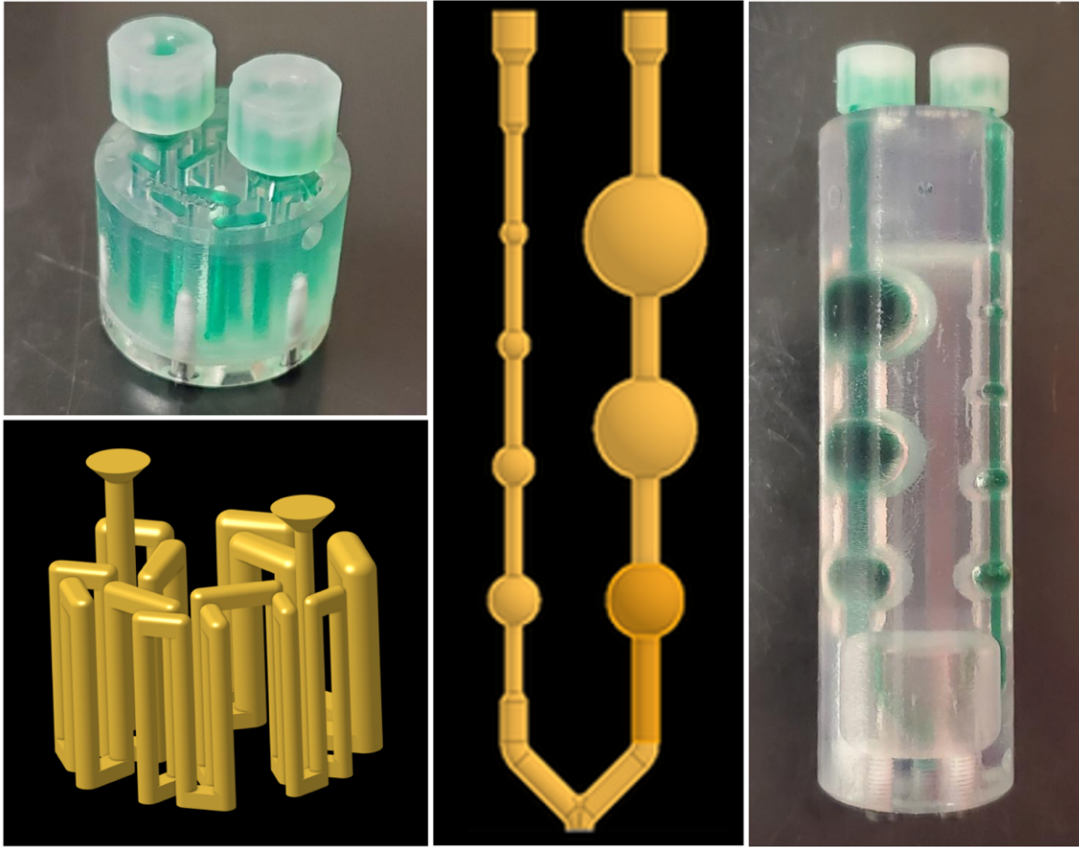
Figure 35: phantoms used for ^{117}\text{Sb} PET and SPECT image characterization. (left top) picture of filled Derenzo phantom (left bottom) CAD drawing of Derenzo phantom channels (middle) CAD drawing of PVE phantom (right) picture of filled PVE phantom.
